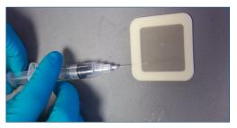
Thorough inspection for salt contamination (including chloride concentration measurement) ensures optimum surface preparation
