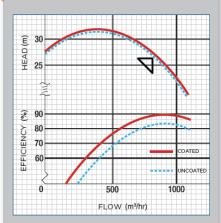
For this test, a single stage, end suction centrifugal pump with 10 inch suction and discharge branches was chosen. In uncoated condition and running at 1300 rpm, the pump was found to deliver  $875m^3/hr$  at 26.5 meter head with an overall peak efficiency of 83.5%.
