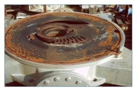
Erosion-corrosion damage on port plate
