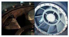
Diffuser vanes with steel gauze in place
