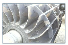
Damaged rotor before rebuilding
