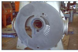
Port plate repaired with Belzona 1111
