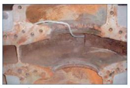
Corroded and cavitated pump
